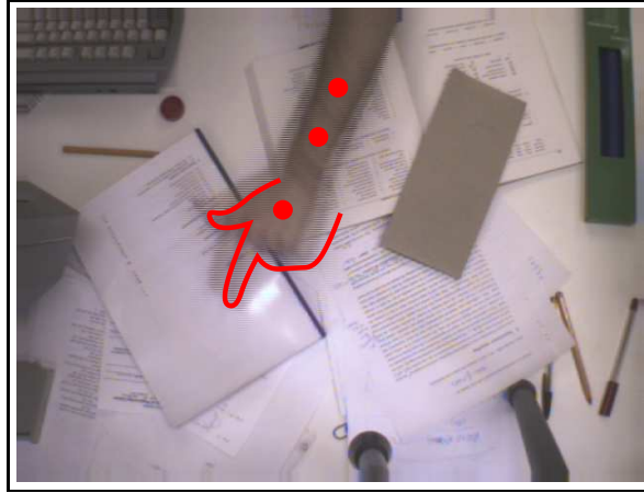
Figure 6.8: Tracking follows high-speed motions. Both fields of a frame are shown, and interlacing artifacts demonstrate the rapid translation of the hand. The tracker is using N=400 samples.
