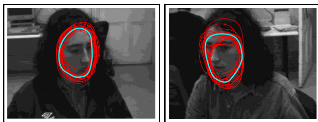
Figure 13: Pose variations A foreground distribution was trained on 3 training images. Test images here show the posterior from broadly distributed priors, under variation of pose.
